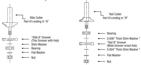
Whiteside Stile & Rail Sets are assembled for traditional door construction using solid wood Raised Panel with 1/4" wide tongue. The Part 6000X Conversion Kit converts these sets to a narrow tongue and groove required for a tighter fit with undersize plywood panels. This conversion is made by switching two groovers of different widths on both cutters. See diagram for details.
